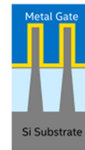
14 nm 2 nd Generation Tri-gate Transistor
