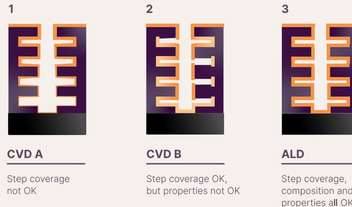
On our XP platform, we offer Pulsar and EmerALD single-chamber ALD process modules for high-k dielectric and metal gate films respectively. The Synergis ALD tool uses the XP8 platform with DCM modules, and leverages the core technologies from our Pulsar and EmerALD ALD products for high-productivity thermal ALD applications. Synergis is available for a range of films, including high-k metal oxides, metal nitrides, and metals.
